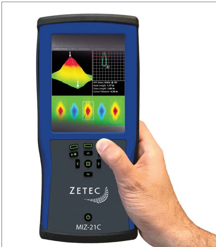
Fig. 1 — Handheld eddy current tools increase test speed and are easy to use. Color touchscreens and C-scan capability provide real-time visual feedback to the technician and the welding crew.
