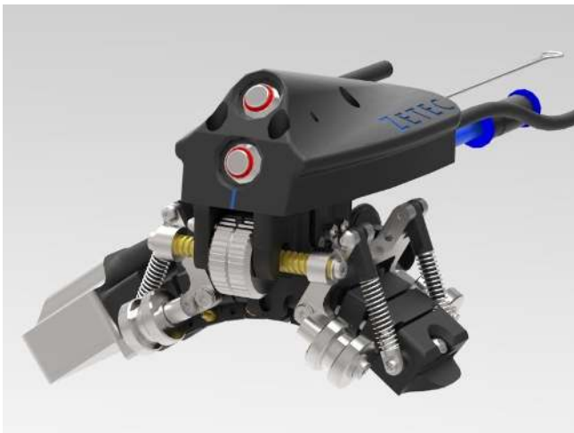
Figure 1. UT scanner for pipe elbows.
