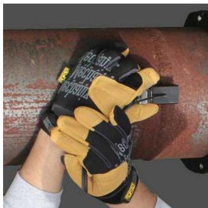
Figure 2. Left: A 1D linear array probe is ideal for most inspections of welds and other defects. Right: The beam-skewing capability of 2D matrix array probes means more accurate wall thickness measurements and better detection of mis-oriented flaws.
