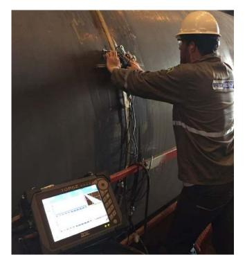
Figure 1. The simultaneous use of phased array UT and TOFD can detect all welding flaw types and provide reliable through-wall sizing in one single inspection. They can produce higher detection capability, more accurate characterisations of corrosion and complete coverage of the material under test.
