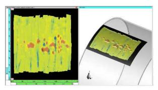
Figure 2. Advanced phased array UT instruments and software can transform 2D scans and CAD drawings into 3D depictions of corrosion damage and other indications. This type of imaging makes test results far easier to communicate.
