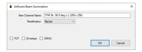
**PCF**: Applies a pixel weighting function based on the coherence factor, which is calculated from the amplitudes of the contributing pulser-receiver A-Scans and is maximized when these are in phase and identical;
