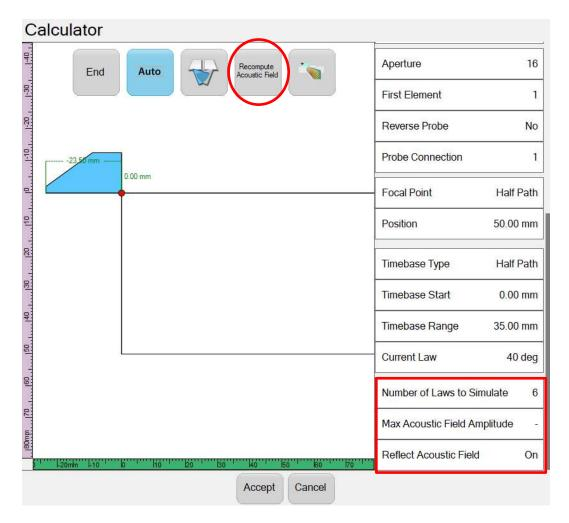
After a parameter change, the acoustic field can be recomputed using the button in the top right of the calculator views. New menu options are also available:
