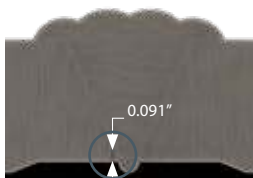
Flaw 3: Root Crack Length: 0.306"
