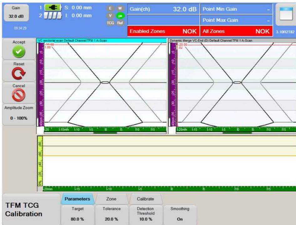
User then can create calibration zones, corresponding to the position of the reflectors. Zones can also be adjusted on the width of the TFM frame:
