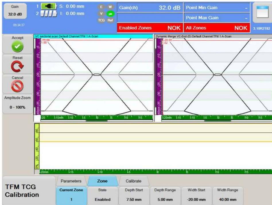
Zones can be computed and calibrated one by one or all together at the user convenience. Once the calibration is completed, user can confirmed zone(s) to have an accepted calibration:
