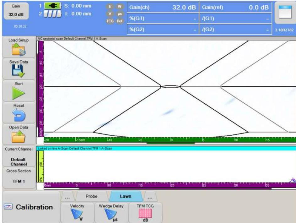
To do the TFM TCG calibration, user first needs to set the target amplitude, tolerance and threshold:
