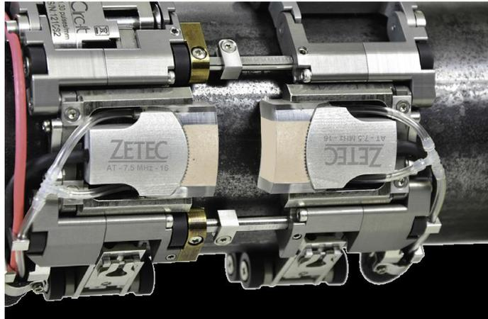
**Circ-it** is a manual small diameter scanner, designed to provide encoded position inspection of circumferential weld around piping and tubing from 21.4mm (0.840in) to 114.3mm (4.500in).
