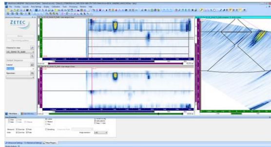
**Volumetric Merge** is an important analysis tool for phased array UT data. An improved interpolation function is now available in Ultravision 3.8R16.
