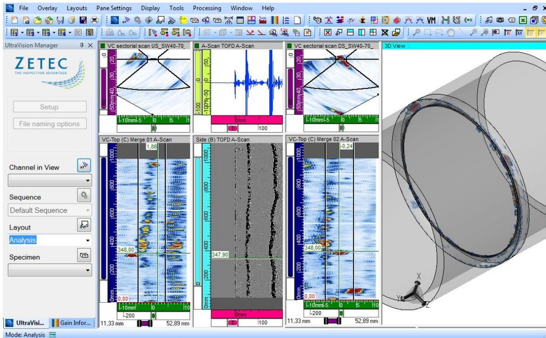
*UltraVision®, a complete UT and Phased Array inspection package!*
