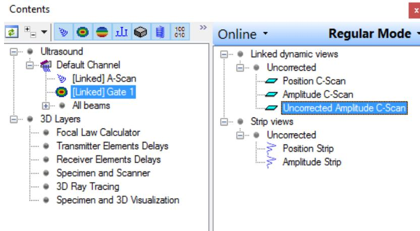
4. Select the gate you want to display this view. Select **Uncorrected Amplitude C-Scan** for this gate.
