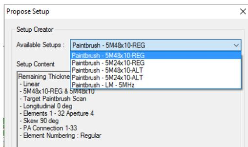
The Propose Setups with regular and alternate probes are an easy way to set up a Paintbrush when using a dual linear array type probe (refer to probe catalog for details). Two probe wirings are available:
