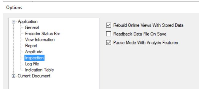
The **Readback Data File On Save** is unchecked by default. When checked, the just-saved data file will automatically open each time you save a copy.
