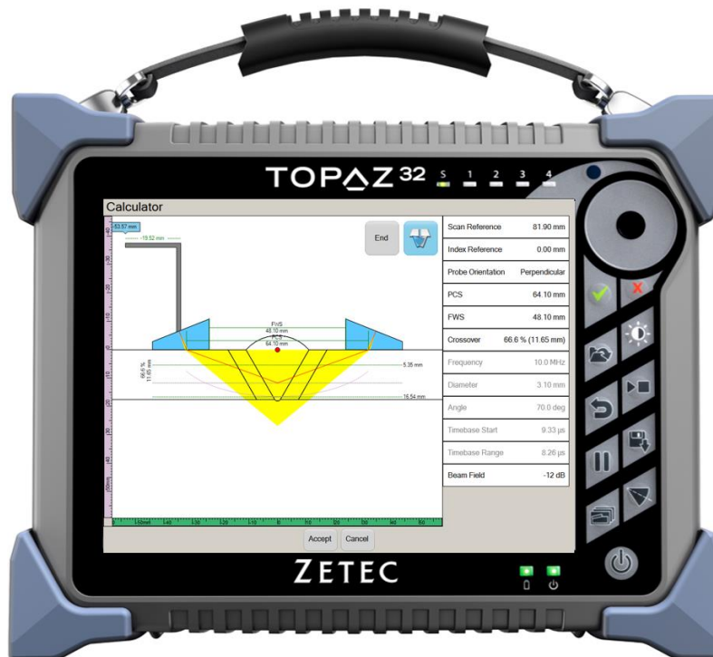
Figure 5: On-board TOFD Calculator
