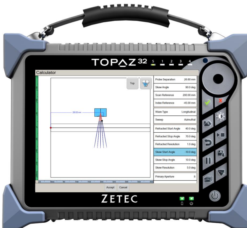
Figure 6: On-board 2D Matrix PA Calculator
