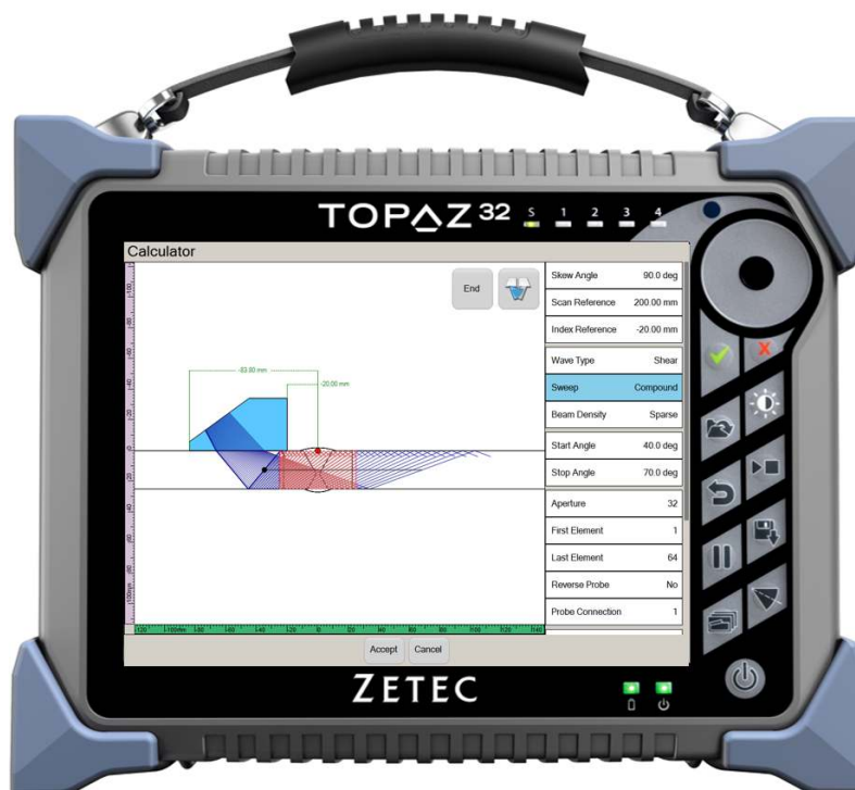
Figure 7: On-board PA Calculator with Compound Scanning Capabilities
