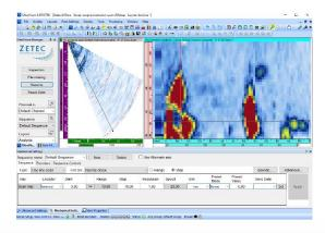
The **Non-Corrected C-Scan View** displays the amplitude readings of each focal law taken from the gate and plotting the information side by side, without correction for actual angle.
